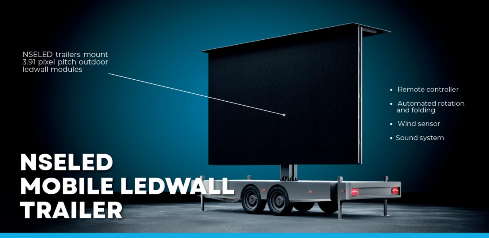
Static calculations and structural analysis are done by engineers from Kaunas University of Technology. NSELED trailers can accommodate LED screens up to 28 square meters and withstand winds up to 15 meters per second.
